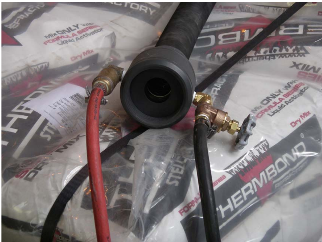
November 2006: Thermbond gunning nozzle assembly for Loy Yang gunning repairs.
