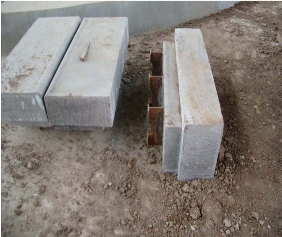
Refractech Pre-cast block design for door lintel and jamb
